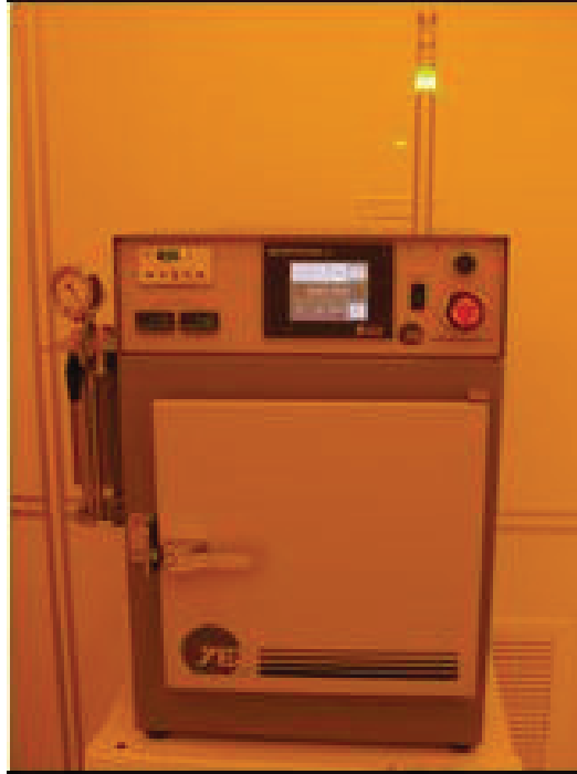
Figure 3.3 YES Image Reversal Oven
