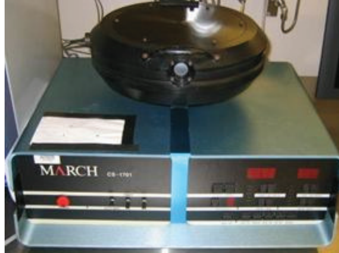
Figure 3.5 March reactive ion etcher (RIE)
